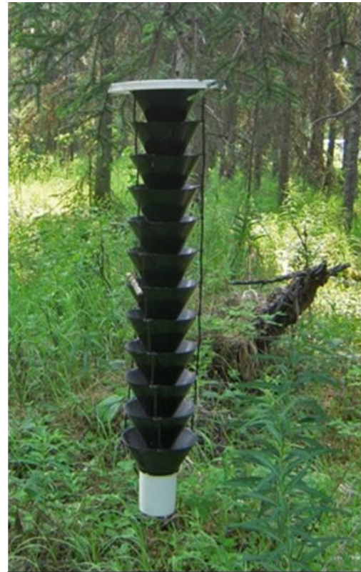
Figure 3: A Lindgren funnel trap, used throughout Mississippi each spring to monitor southern pine beetle populations.
